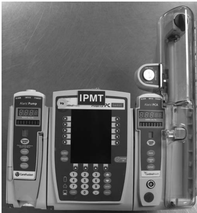
Figure 17-17. Alaris Smart Pump for controlled intravenous medication administration. (Courtesy of William Salkin.)
